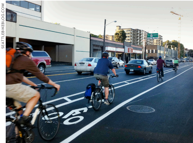
This buffered bicycle lane on Dexter Ave N offers increased space and more comfortable separation from moving vehicles than a conventional bicycle lane.
